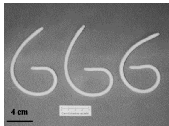
Fig. 10. Photo images of boehmite tubes showing the repeatability of making bend tubes using the developed extrusion technique.
